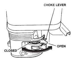
Figure 13. Choke Lever
